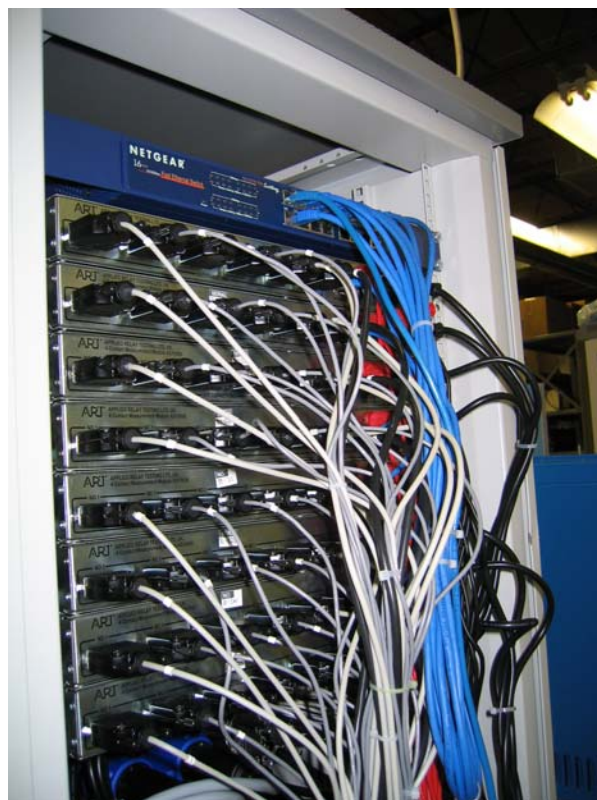
Figure 4 – Ethernet connections carry TCP/IP at the rear of the Reflex 50 life-test system.
