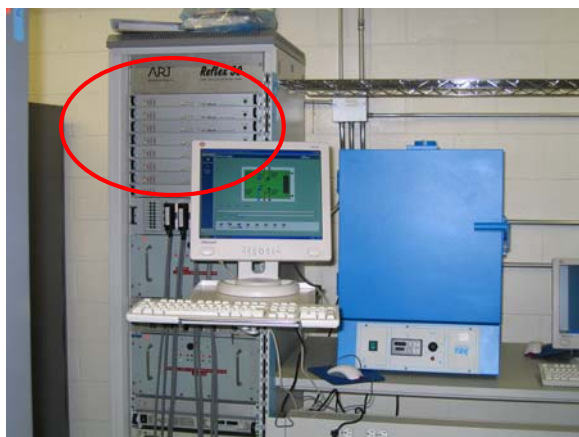
Figure 3. A TCP/IP connected solution - the Reflex50 life-test system.
